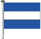
( I am on fire and have dangerous cargo on board: keep well clear of me, or I am leaking dangerous cargo.
