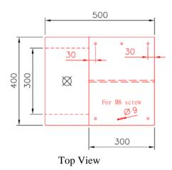
(p) The bottom and top flanges of vertical unit shall be with bolt hold pattern (in mm) presented as follows:
