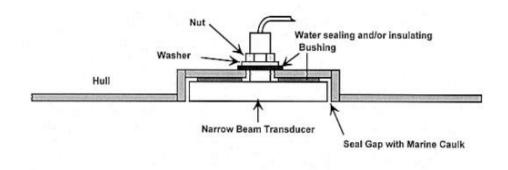
Transducer must be flush with hull
