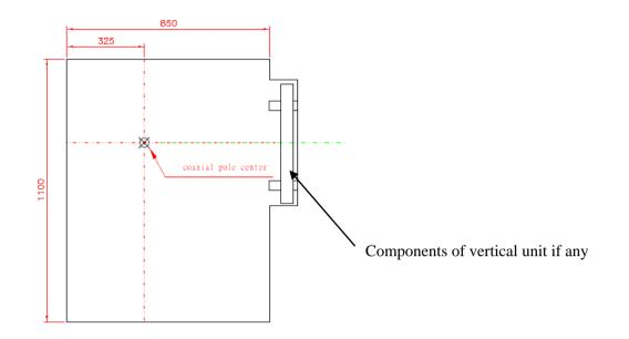
The lifting appliance shall be fixed outside the moon pool or in a position not affecting the vertical movement of the coaxial pole with MBES transducer installed. The whole system shall meet the following requirements, unless otherwise specified: -
