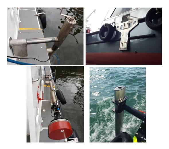
4.16.11A moon pool with 1.1m x 0.85m opening shall be located nearby the COG of the vessel. A vertical unit equipped with a lifting appliance shall be fixed at the aft centre next to the toilet for lifting and lowering of vertical unit into and out of water. The vertical unit shall comprise of a coaxial pole which allow a Multibeam Echo Sounder (MBES) transducer installed at the bottom and 3 GNSS antennas & a lasers scanner installed at the top. [E]
