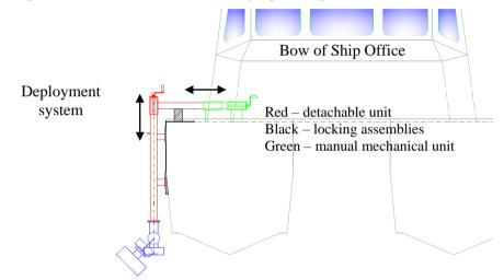
With the two directions manual extension mechanisms, the side mount shall be able to move in up-down and port-starboard directions. It allows the sonar transducer pole to be deployed from deck level into the water smoothly and vice versa. The side mount system shall meet the following requirements, unless otherwise specified: -
