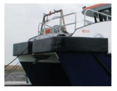
4.13.3 Additional Rubber Tyre Fenders at Bow and Ship's Sides:
