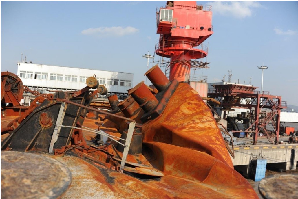
Dent of Bow from Starboard to Portside
