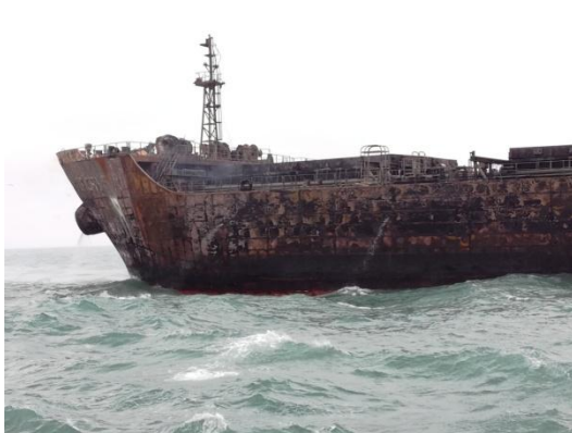
The damage to the bow of CF CRYSTAL and color difference between bow and midship
