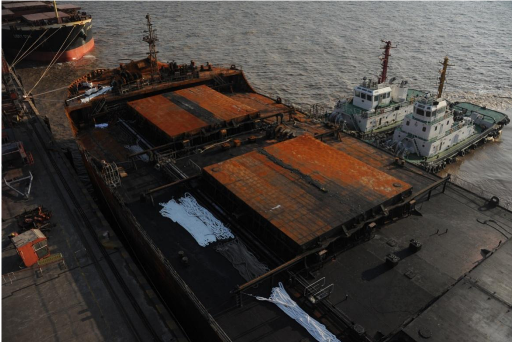
Top View from Midship Forward (forward No.3 cargo holds sustained fire)
