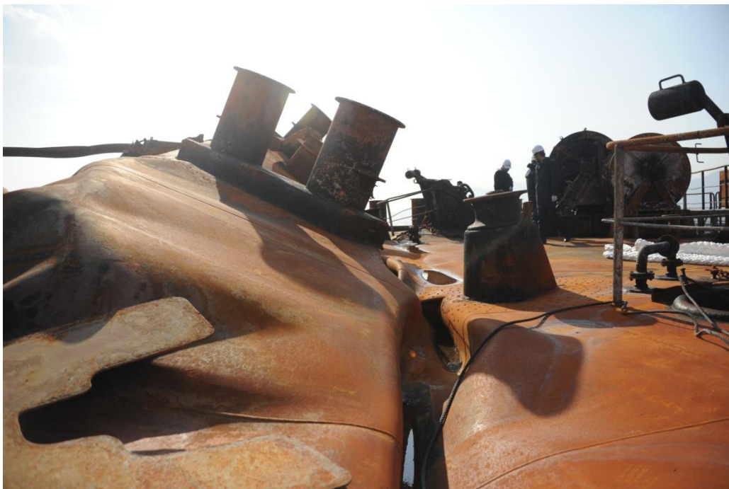
Forecastle deck bending backwards
