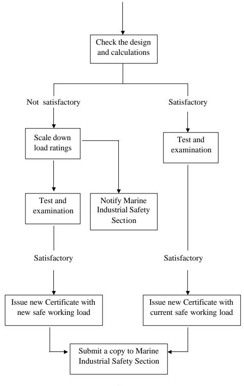
Case 2: Derrick cranes with current Certificate of Test and Examination but the drawings/calculations are not available or incomplete
