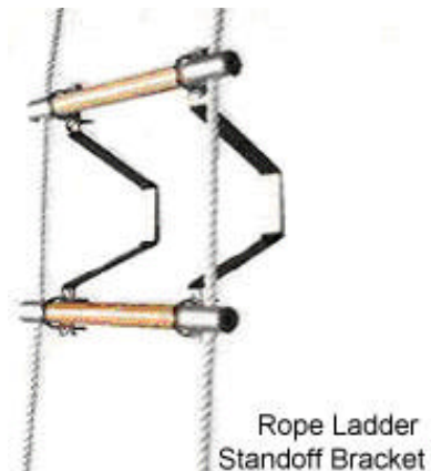
Photo 8 – Rope ladder with standoff bracket to provide sufficient space (at least 115mm) for footholds
