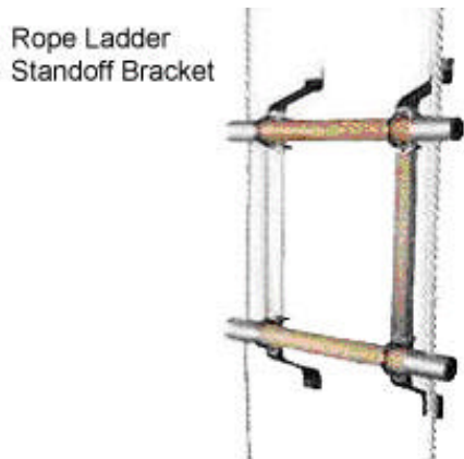
Photo 8 – Rope ladder with standoff bracket to provide sufficient space (at least 115mm) for footholds
