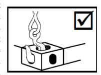
5.2.911 If there is any possibility of jamming containers in cell guides, hook slings should not be used to lift or lower containers through cell guides. Suitable equipment such as spreaders or slings with special lifting keys should be used. Never attempt to lift containers
