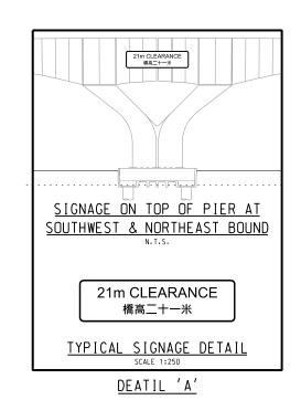
THE LAYOUT OF NAVIGATION SPAN AT TM-CLKL AREA NO. 1
